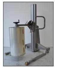
for heavy roles allows rolls to be lifted and swiveled with a side gripper
