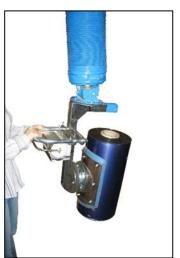
90 ° rotating device for erecting or laying down rolls
