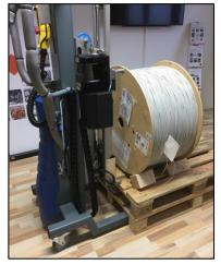
cable reels combined with an electronically operated gripper
