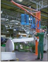
double hose for lifting heavy rolls
