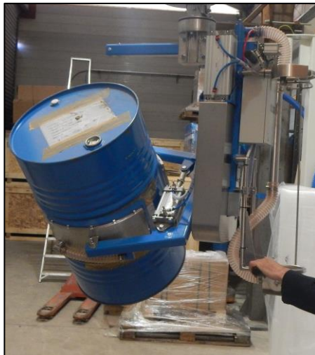
vacuum lifter with side holding of barrels with lifting and tilting device
