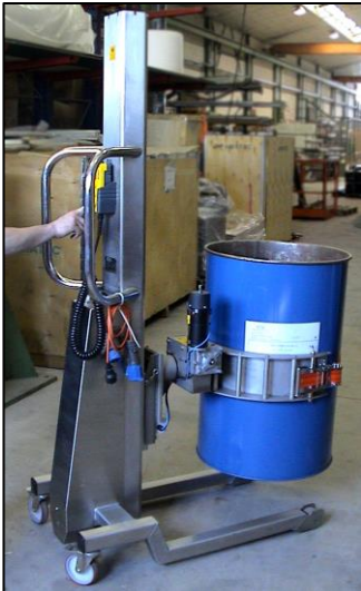
lifter with side receptacle for barrels to grip and rotate
