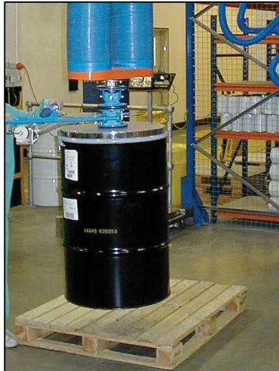
sucker for picking up barrels from above
