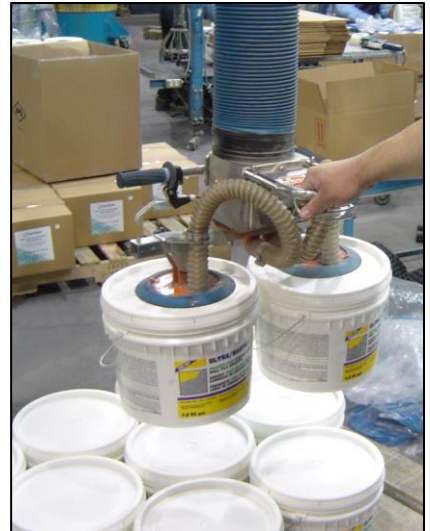
vacuum lifter with double suction cups for lifting several containers
