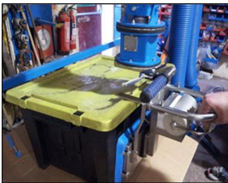
vacuum lifter with angled suction cup for lateral lifting of KLT boxes with loose lids
