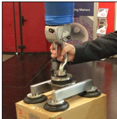
vacuum lifter with one-hand operation for lifting cardboard boxes up to 50 kg.
