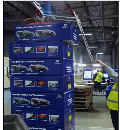
vacuum lifter with extended handle for a stack height of up to 2.5 m
