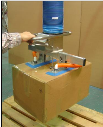
vacuum lifter with adjustable suction cups
