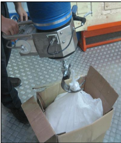
vacuum lifter with a special gripper when pulling plastic bags out of a cardboard box
